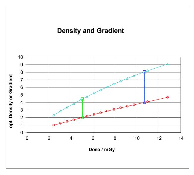
**Figure 1:** Mean optical density <D- $D_0>$  (red curve) and mean gradient <G> (blue curve) of eight films as function of exposure dose K.
